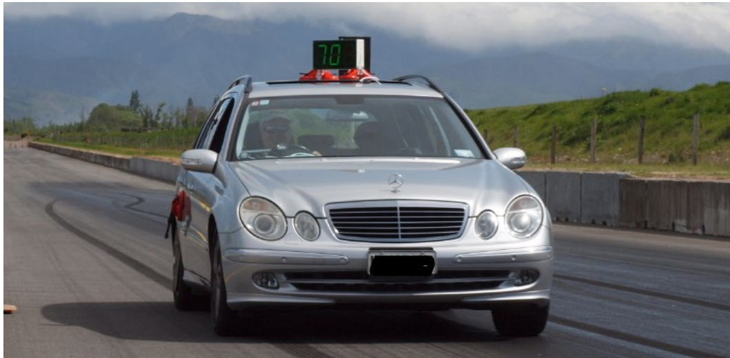
Sighter board display on test vehicle
