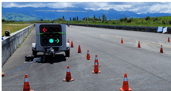
HALO Red-light /speed system set up
