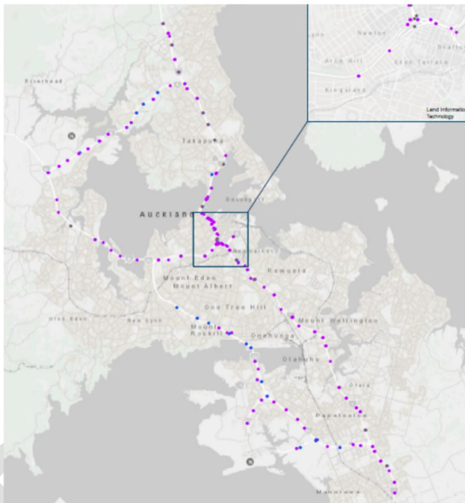
AT has a limited number of cameras being used with a VMS based ANPR solution to enforce special use lane compliance (bus only lanes). It is also used for measuring journey times by recording the time for unique vehicles to travel between fixed locations.
