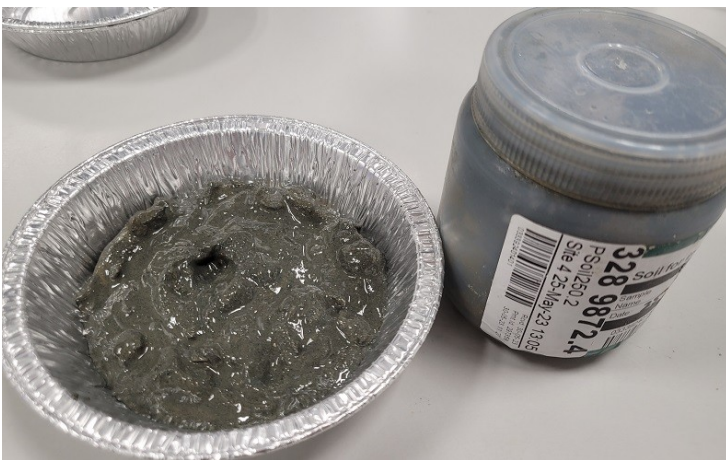
Sample 5.09 - 3289872.4 – contains a lot of small univalve shells, periwinkles, pieces of shell and mud
