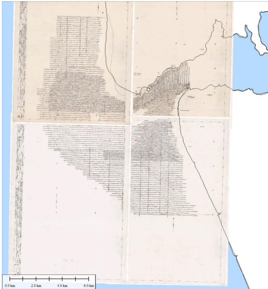
Figure 3-1 LINZ scanned sounding sheets number 4314 – Manukau Harbour mouth 1989.
