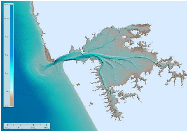
Figure 1: Final bathymetry dataset (bar region based on 2023 survey data (DML 2023)).
