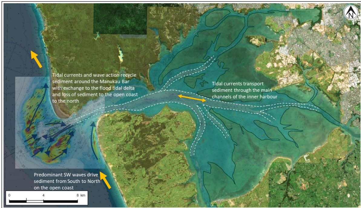
Figure 4.7: Simplified conceptual model of sediment transport around the Manukau Harbour.
