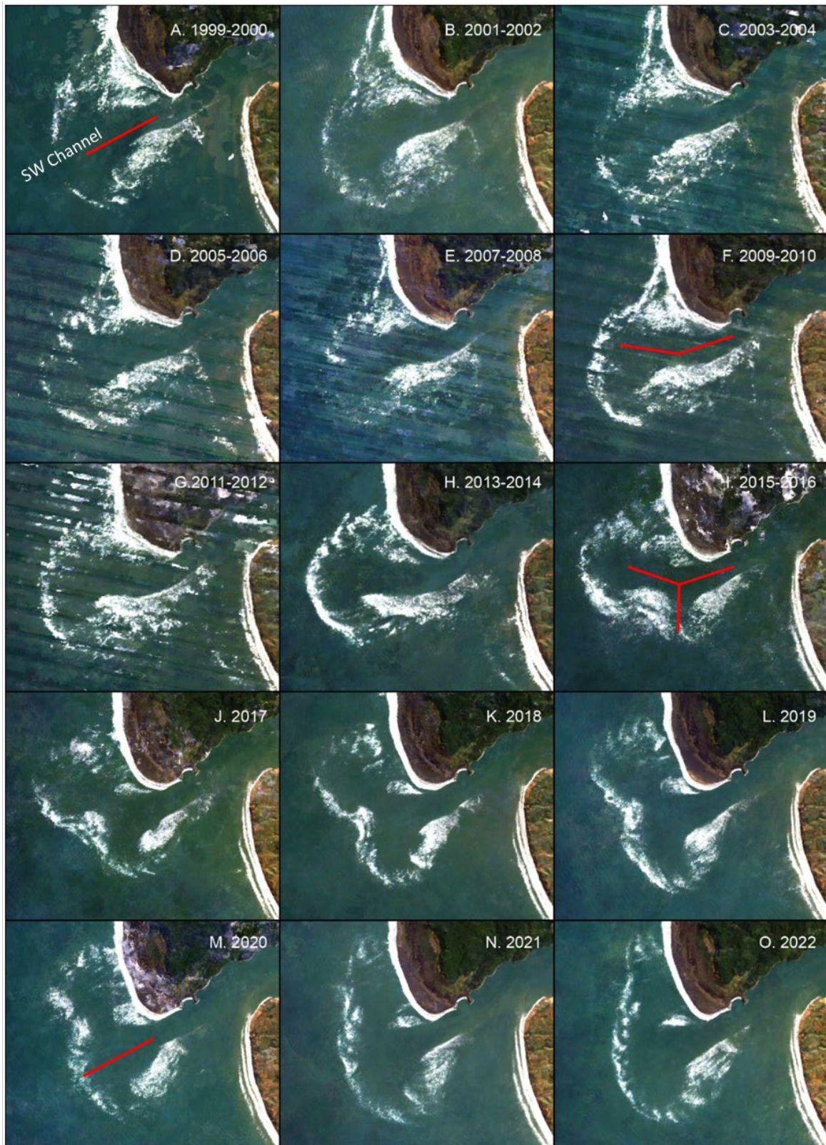
Figure 4.2: Satellite imagery of the Manukau Bar over time indicating a gradual migration of the main SW channel to the north (2009 to 2015) before a channel bifurcation starting in 2015 and re-establishment of a main SW channel around 2019-2020, as indicated by the red lines.
